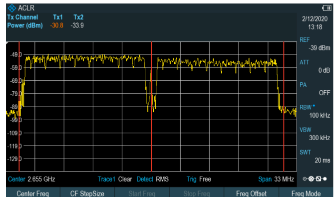
Gated trigger in ACLR mode with the R&S®FPH-K57 advanced gated trigger measurements option
